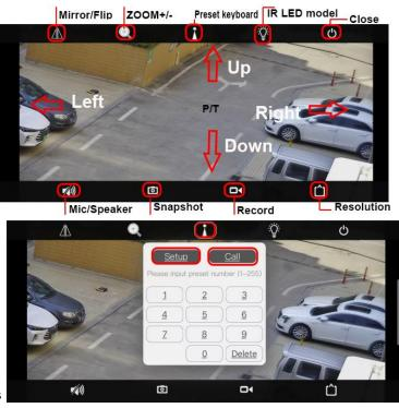
to the return position and continues to wait for the next tracking. The return position is 88<sup>th</sup> preset.please set 88<sup>th</sup> preset Call 97 for Turn on tracking, Setting method: [97]+[Call]; set 96 for turn off tracking, Setting method: [96]+[Set]
